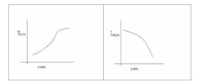
**<u>DISCUSSION</u>**: - The graph is plotted between speed and torque. As we reduce the speed of the motor the torque goes on increasing therefore the graph starts with a low value and rises to a high value approximately linearly .This rise in the graph is due to the rising speed- torque characteristics of AC servo motor.
