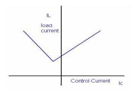
$\underline{\text{DISCUSSION}}$ : - The graph is plotted between control current(IC) and load current (IL)For positive polarity the control current increases linearly with load current in forward Direction but for negative polarity the control current increases load current in reverse direction. This change in direction of control current is due to change in polarity of control voltage.
