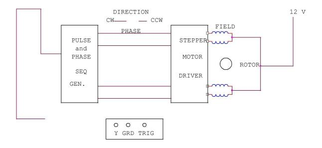
**PROCEDURE:** Connect the stepper motor with µp 8085 kit as shown in fig. press EXMEM key to enter the address as given then press NEXT to enter data
