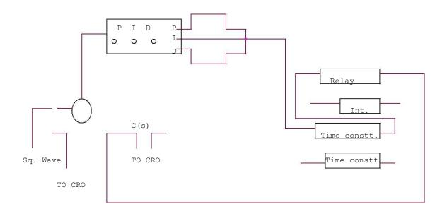
**PROCEDURE** : P control mode: connect the circuit as shown in the figure. Switch over CRO for XY mode. Adjust P control to 0.1 and note the X and Y values. Increase the value of P and note the results in table. Input 1.0 Vpp , squire wave of 50ms . I not connected to adder and D control at 00. switch over CRO in tigger mode and find out period of oscillation. Switch over again in XY mode and find out percentage over shoot and steady state error
